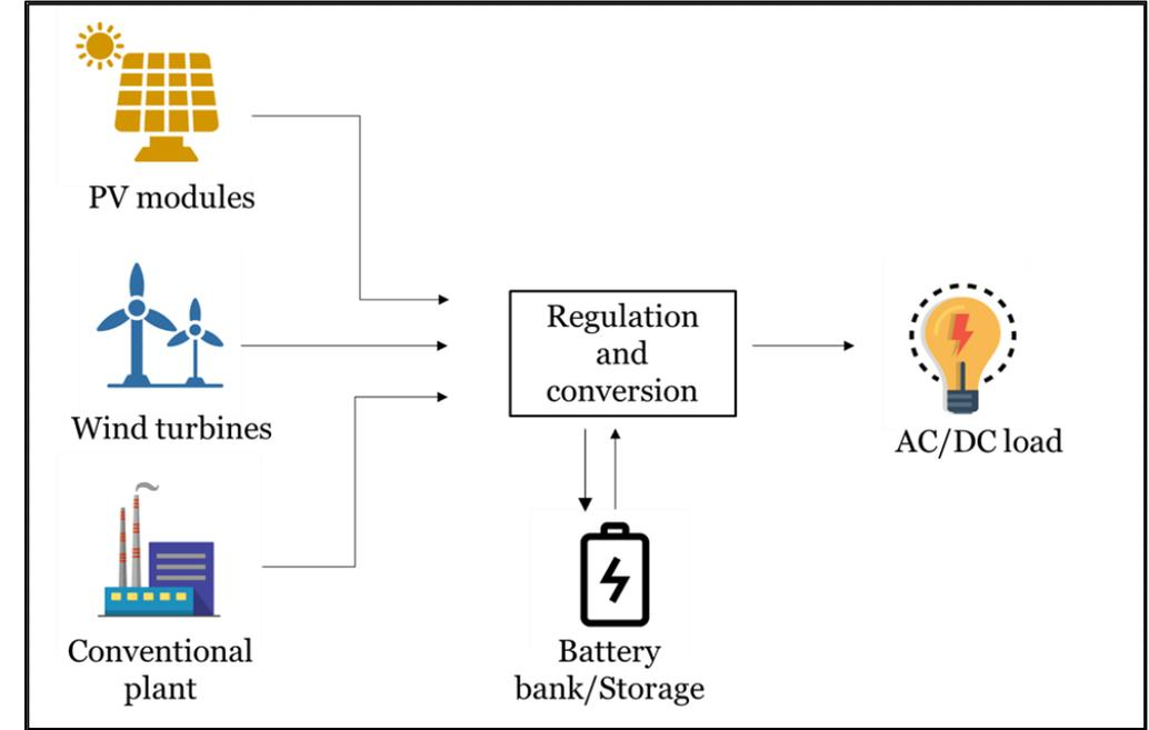
Fig. 11: Hybrid Power Plant
