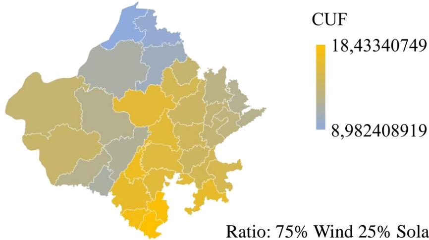
Capacity Utilisation Factor of Hybrid PV-Wind Plant
