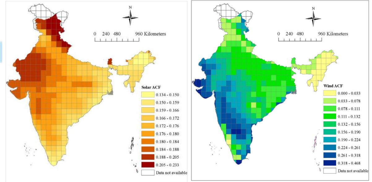
Fig. 8: Annual capacity factor for solar PV plants and on-shore wind plants
