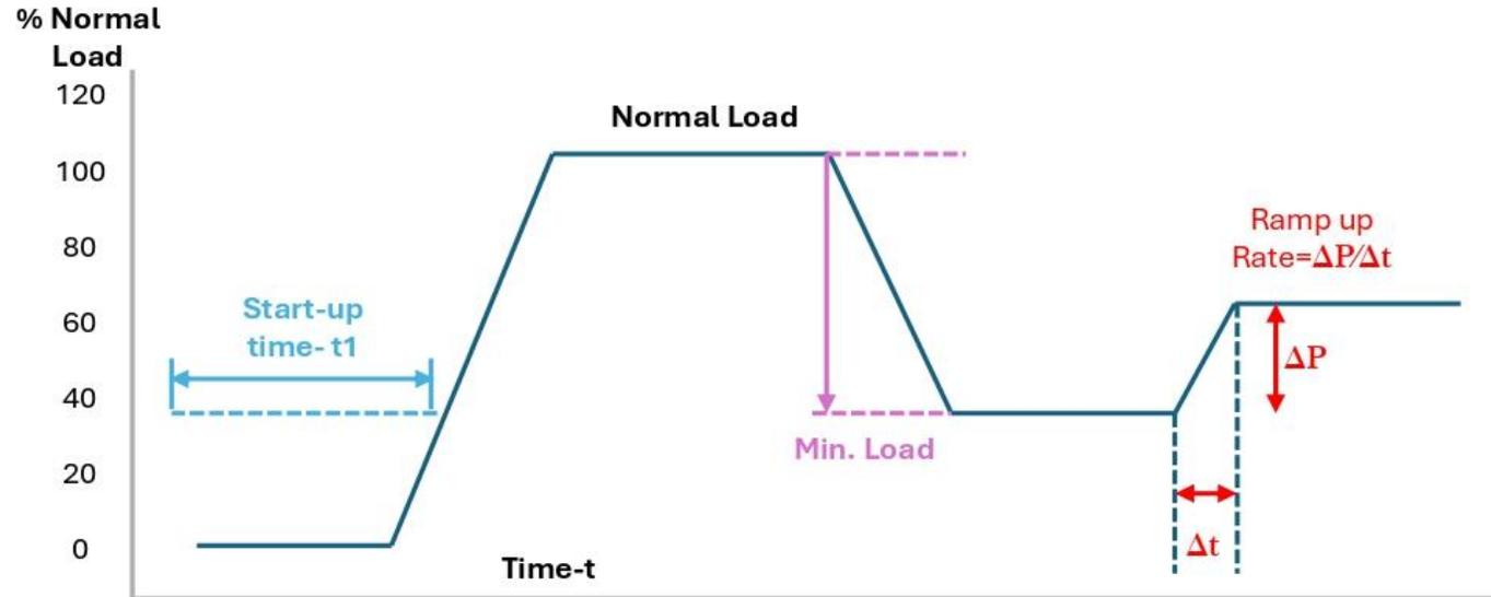
Fig. 10: Attributes of Flexible operation
