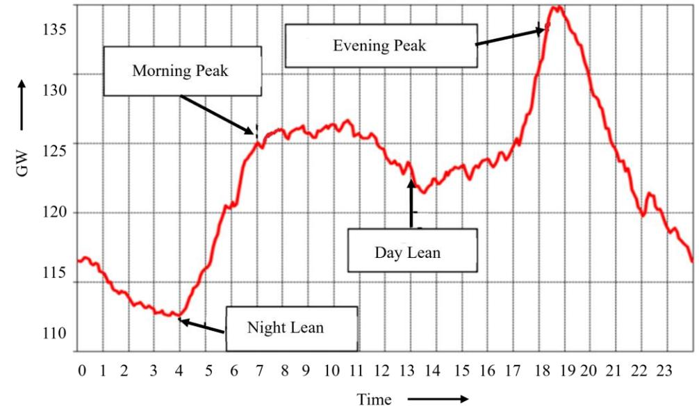
Fig. 5: load curve
