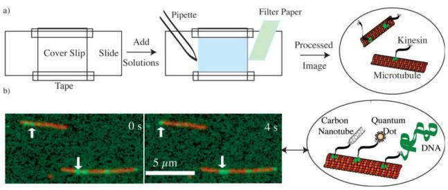
Fig. 1. **a:** Flow cell formed from a microscope and a slide separated by double-sided tape. Different solutions are perfused into the system by capillary forces. The flow cell system is used to transport kinesin on immobilized microtubules tracks. **b:** Proof of principle: green fluorescent protein (GFP) kinesin walking on the microtubules.
