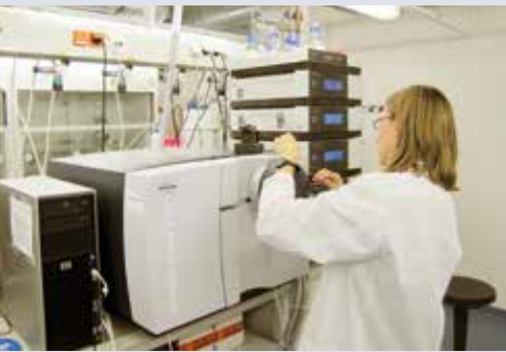
▲ Using an HPLC-coupled mass spectrometer (left), we can separate and identify the components of the underwater glue of diatoms (indicated by arrows in the small image top right).
