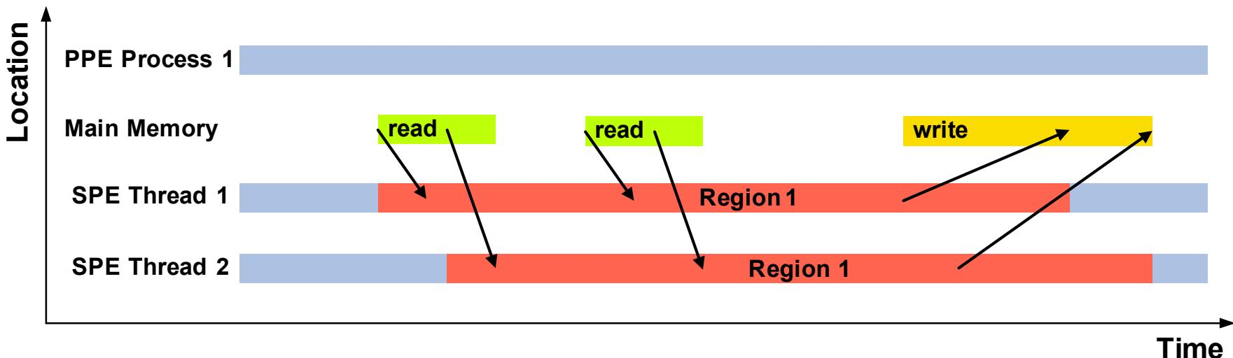
Illustration of DMA transfers between SPEs and main memory
