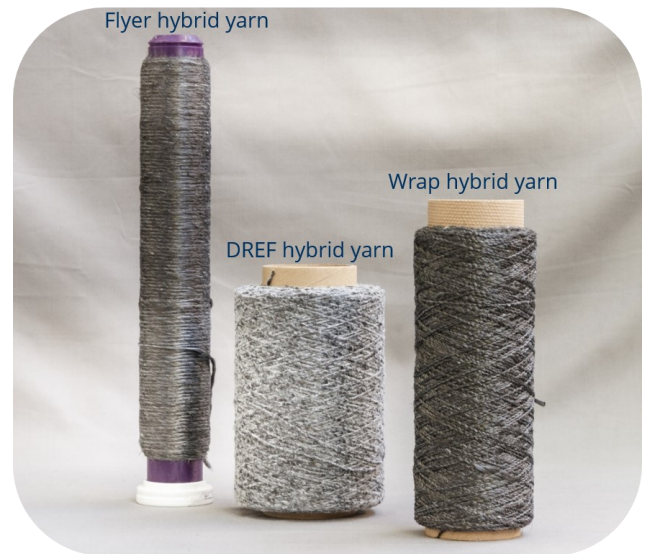
Figure 2. Different rCF hybrid yarns developed at the ITM; source: ITM
