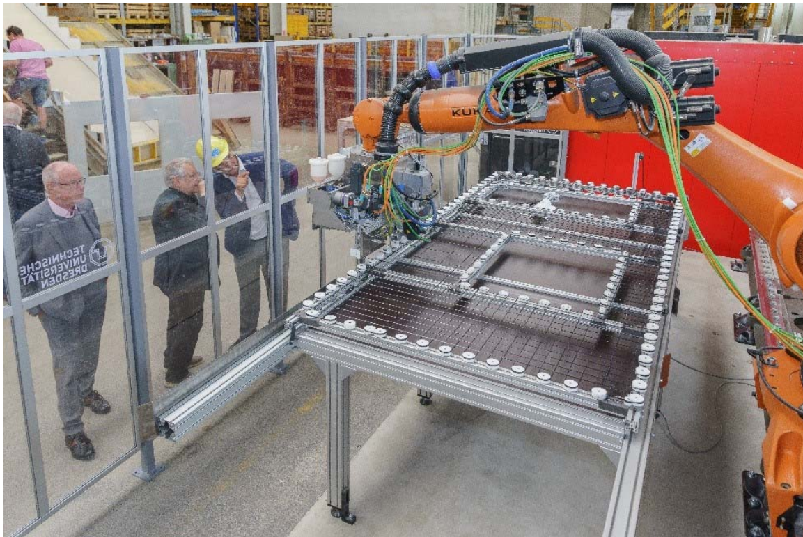
Figure 1: Robot-supported yarn placement technology for the production of cost-efficient carbon concrete precast elements; source: Rico Pöschel (ITM)
