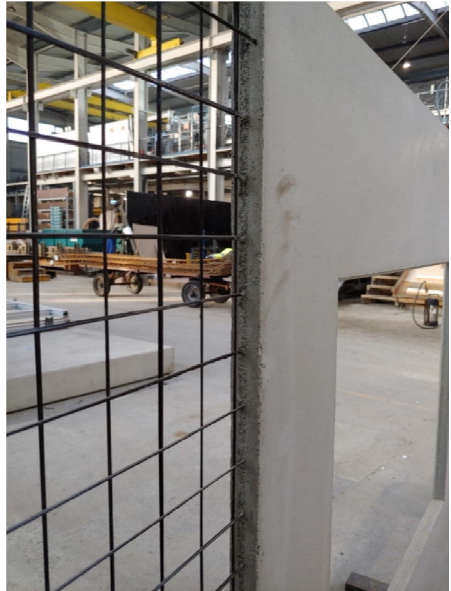
Figure 2 Cost-effective wall element with openings consisting out of carbon fibre reinforced concrete; source: Martin von Zuben (former: ITM)
