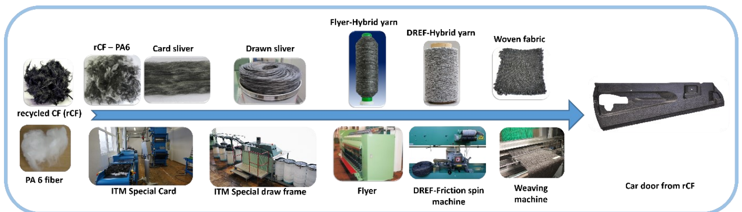
Figure 1. Process chain for the manufacturing of fibre reinforced composites from rCF Hybrid yarns at the ITM; source: ITM
