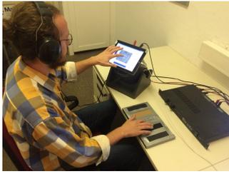
**Figure 3:** The subject tuning the frequency and amplitude ratio using the experimental setup. The experimental setup includes textures, shaker, amplifier and iPad as seen above.
