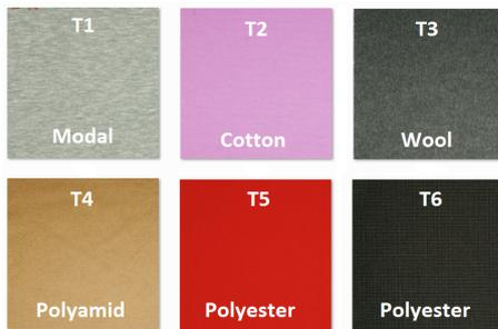
**Abbildung 1:** Fabric textures are sorted from T1 (finest) to T6 (roughest) based on their spatial density and subjective roughness evaluation test. Types of the fabrics are written as above.
