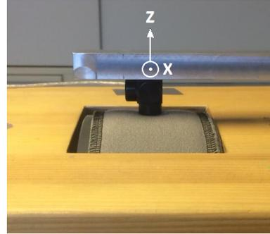
**Abbildung 2:** Acceleration measurement setup. Rotating drum provides relative motion between texture and contacted accelerometer.
