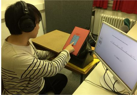
**Abbildung 4:** The participant is touching haptic display and textures which are under the cover in order to rate the similarity. The user-computer interface, texture cover, tactile display, electro-dynamic shaker, and headphone were placed as in the image.
