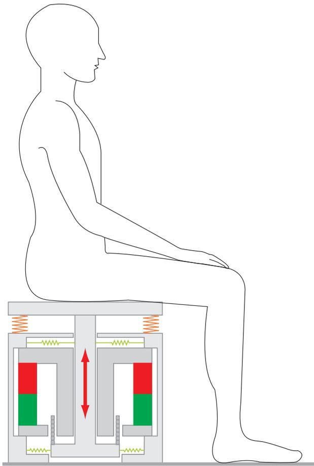
Figure 1. Vibration chair with electrodynamic exciter.
