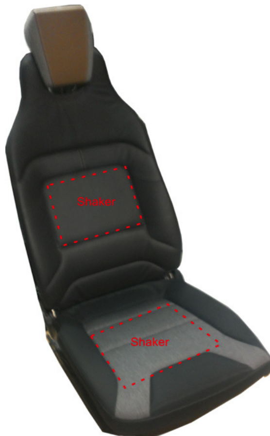
Figure 1: Car seat with the position of electro-dynamic shakers.
