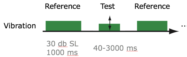
Figure 4 – Experimental procedure: the reference and test vibrations were presented in alternation until a participant was satisfied with her/his intensity matching. The amplitude of the reference stimulus was fixed at a level of 30 dB above the threshold. The amplitude of the test stimulus could be adjusted.
