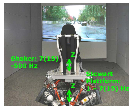
Figure 1. The tactile stimuli described in section II were presented on the depicted whole-body reproduction system (with frequency range for low sensation level (and high sensation level)) For the presentation of audio visual tactile scenes also audio and video were presented.
