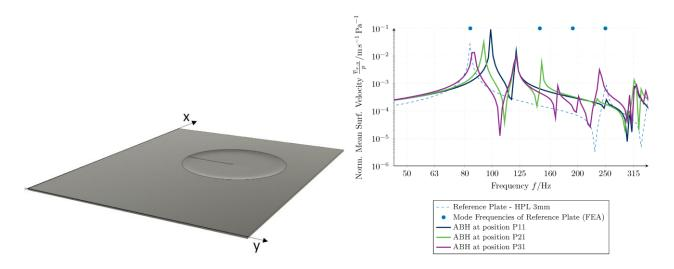
An acoustic black hole (ABH) is a power-law tapered profile that reduces wave propagation velocities to minimal levels. ABHs have been effectively applied in engineering structures for noise and vibration control.
