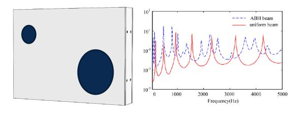
Acoustic black holes (ABH) have been successfully employed for controlling noise and vibrations in mechanical structures. An acoustic black hole is a power-law tapered profile on a structure to decrease velocities of wave propagation to minimum levels.
