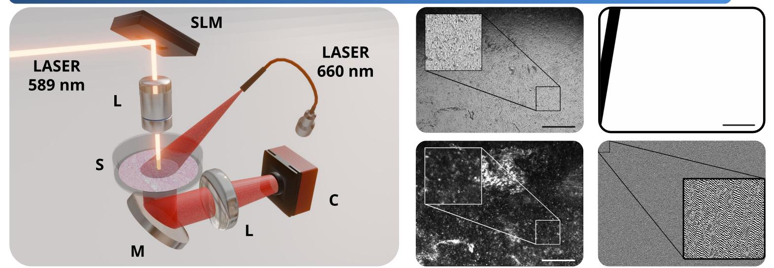
Left: Simplified scheme of the optical setup for holographic stimulation (orange path) and label-free imaging (red path) of the hiPSC-CMs; components: SLM spatial light modulator, L lens, S sample, M mirror, C camera. Center: Widefield (top) and speckle image (bottom) of the same cardiac monolayer. Right: Stimulation pattern (top, illuminated area visualized in black) and respective hologram (bottom). Scale bars: 2 mm.
