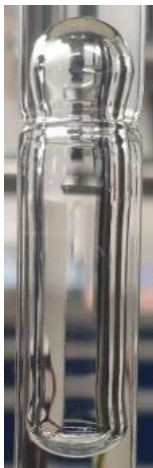
Fig 1: Taylor bubble in glass tube with constriction
