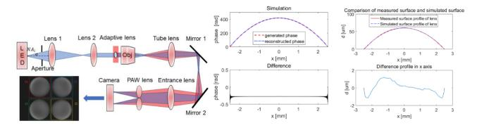
PAW imaging device in a Köhler illumination (left), the reconstructed phase shift induced by a simulated lens (middle) and the reconstructed phase shift of a fix lens in experiment (right).
