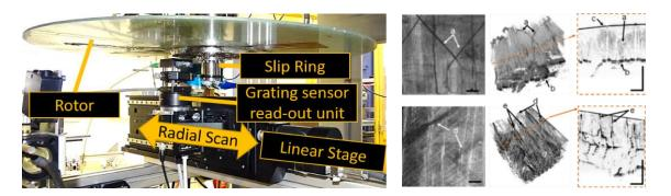
Diffraction Grating Sensors measuring in- and out-of-plane FRP rotor deformation field and vibration at >270 m/s with 20  $\mu$ s and 15  $\mu$ rad precision (left). OCT images of internal FRP rotor structure, showing delamination (b) and cracks (e) (right) due to overload.
