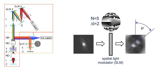
Left: Schematic of setup for simultaneous 3d targeted single cell stimulation and single shot 3d localization microscopy. Right: Principle of 3d localization microscopy with point spread function engineering. Single image points are converted to double spots using a special phase mask in fourier space. The depth of the light source can be estimated from the orientation angle  $\psi$  between the double spots which changes along the optical axis.
