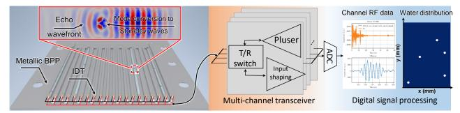
Schematic of the proposed measurement system. Pulse-echo-localization of water droplets is condected by means of surface acoustic waves and a transducer array.
