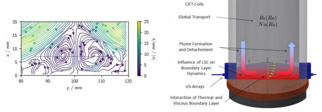
Super-resolution vector flow imaging of a recirculationProjected convection experiment for thermal and viscosearea in a liquid metal convection.boundary layer measurements.
