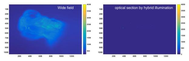
Left: Wide field fluorescence measurement of zebrafish larvae. Right: After spatial frequency analysis, the strong auto fluorescent background is removed.
