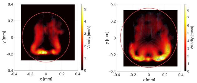
Vector plots of the flow field of a hydrogen bubble growing at a microelectrode with an applied potential of -7 V. The left picture shows the flow at 60 % of the growing time, the right picture right befor detachment. The circles indicate the shape of the bubble.
