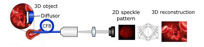
The 3D object is encoded by a diffuser to a 2D speckle pattern which is transmitted through a CFB to a camera. The 3D object is then reconstructed by a neural network.
