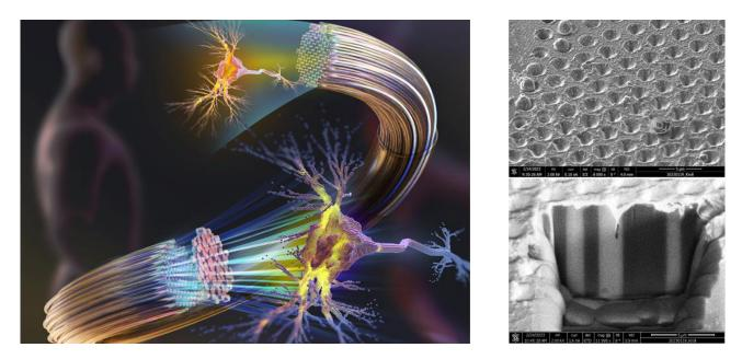
Left: Sketch of a Holographic 3D fiber bundle endoscope. A diffractive optical element is used to compensate the inherent phase scrambling of the fiber. Right: SEM image of an fiber facette after laserablation for DOE manufacturing.
