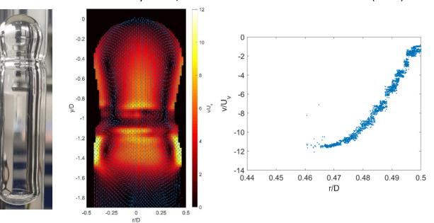
Left: Picture of a Taylor bubble inside a constriction, Middle: Gas flow field of the Taylor bubble head. Right: Liquid film flow velocity profile directly below the constriction measured with double-helix particle tracking velocimetry.
