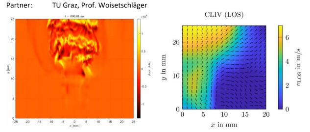
Left: Time resolved densitiy derivative measured line-of-sight in a swirl-stabilized flame. Right: Integral mean velocity, calculated from the line-of-sight density measurement using PIV signal correlation.
