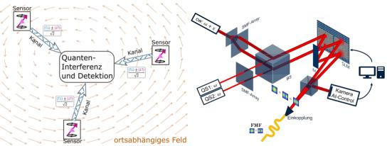
Left: Concept of spatially distributed quantum sensing as an IoT network service. Spin qubits serve as sensors, which transmit the quantum information in the form of photons superimposed at a central server. Right: envisaged approach to translate distributed quantum signals (QS) to a superposition of modes using an SLM and multiplane light conversion.
