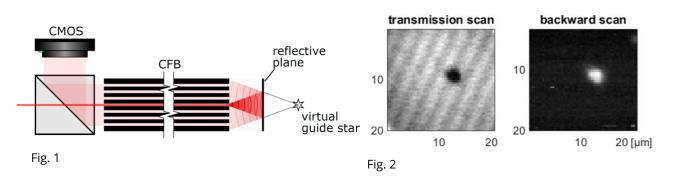
Left: Scheme virtual guide star calibration. Right: Endoscopic scan of fluorescent particle with diameter of 1 µm.
