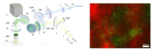
Left: Schematic of a holographic illumination setup for the simultaneous stimulation and inhibition of optogenetically altered cells. Right: Sample image of a cardiomyocyte cell culture (red) overlaid with temporally resolved contraction strength (green) passing over the sample in waves.
