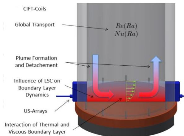
Super-resolution vector flow imaging of a recirculation area in a liquid metal convection.
