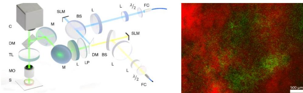
Left: Schematic of a holographic illumination setup for the simultaneous stimulation and inhibition of optogenetically altered cells. Right: Sample image of a cardiomyocyte cell culture (red) overlaid with temporally resolved contraction strength (green) passing over the sample in waves.
