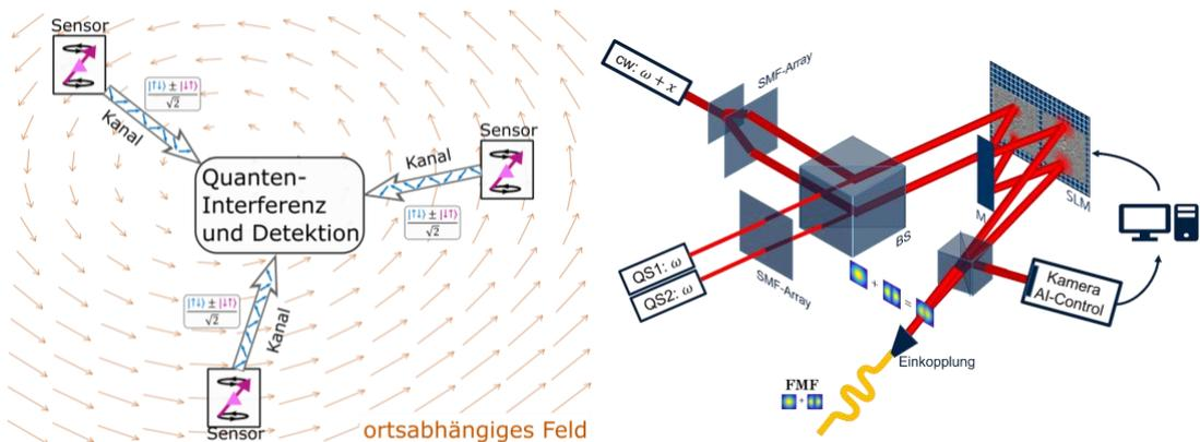
Left: Concept of spatially distributed quantum sensing as an IoT network service. Spin qubits serve as sensors, which transmit the quantum information in the form of photons superimposed at a central server. Right: envisaged approach to translate distributed quantum signals (QS) to a superposition of modes using an SLM and multiplane light conversion.
