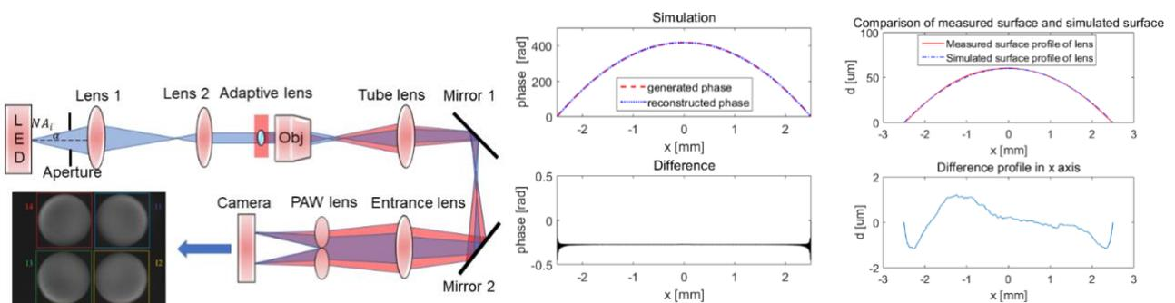
PAW imaging device in a Köhler illumination (left), the reconstructed phase shift induced by a simulated lens (middle) and the reconstructed phase shift of a fix lens in experiment (right).
