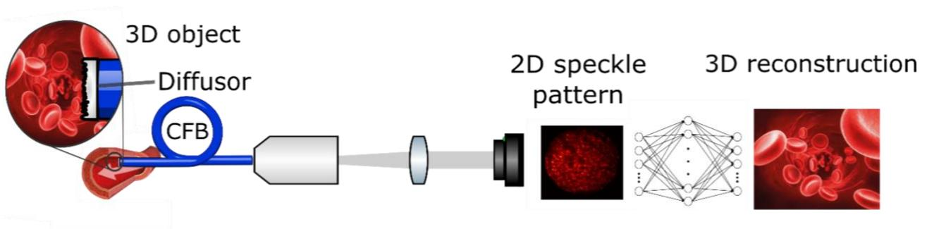
The 3D object is encoded by a diffuser to a 2D speckle pattern which is transmitted through a CFB to a camera. The 3D object is then reconstructed by a neural network.
