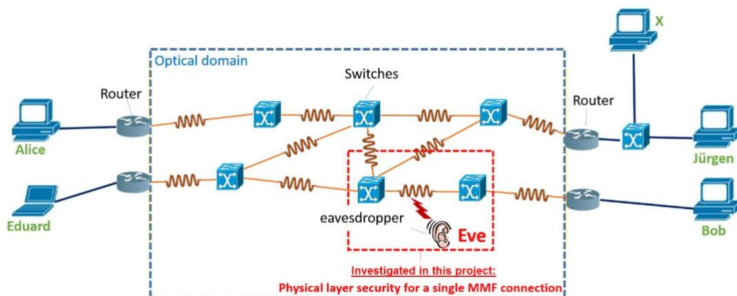
Optical network. In this project together with our partner, the physical layer security for a single MMF connection between two network nodes is investigated.
