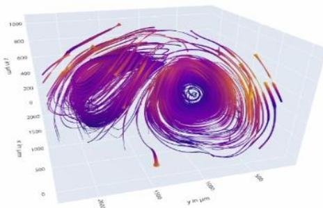
*A grazing flow induces a complex flow pattern in droplets which was measured three-dimensionally for the first time in this project. The tilt of the vortex pairs could be resolved experimentally for the first time.*
