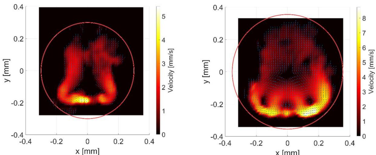
Vector plots of the flow field of a hydrogen bubble growing at a microelectrode with an applied potential of -7 V. The left picture shows the flow at 60 % of the growing time, the right picture right before detachment. The circles indicate the shape of the bubble.
