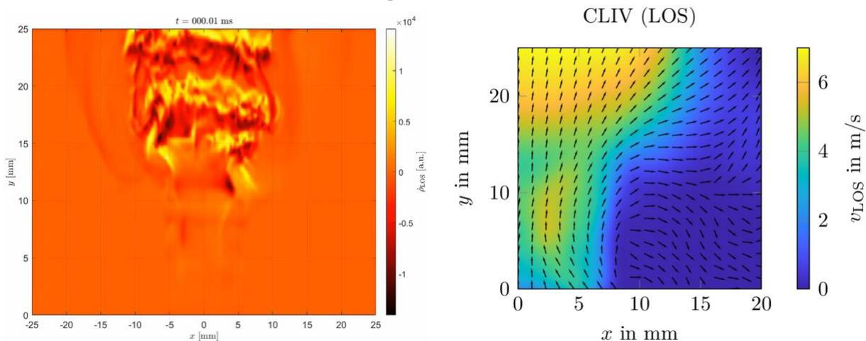
Left: Time resolved density derivative measured line-of-sight in a swirl-stabilized flame. Right: Integral mean velocity, calculated from the line-of-sight density measurement using PIV signal correlation.
