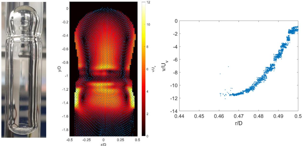
Left: Picture of a Taylor bubble inside a constriction, Middle: Gas flow field of the Taylor bubble head. Right: Liquid film flow velocity profile directly below the constriction measured with double-helix particle tracking velocimetry.
