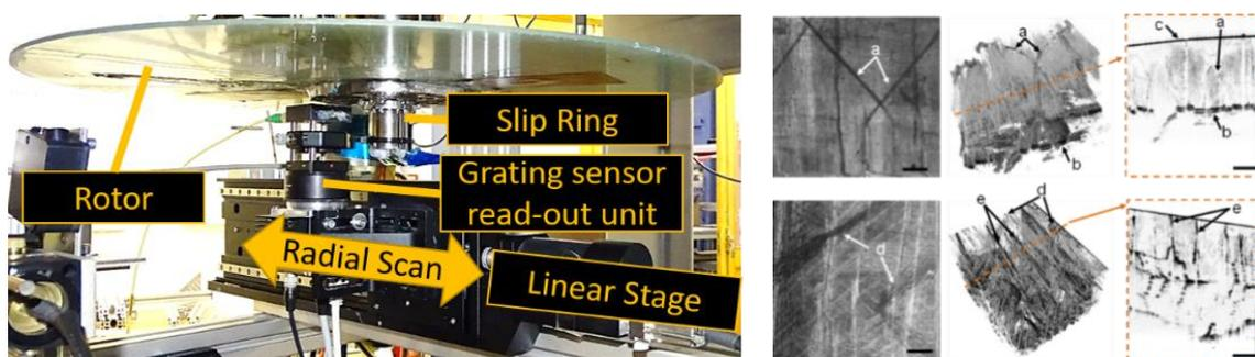
Diffraction Grating Sensors measuring in- and out-of-plane FRP rotor deformation field and vibration at >270 m/s with 20  $\mu\text{e}$  and 15  $\mu\text{rad}$  precision (left). OCT images of internal FRP rotor structure, showing delamination (b) and cracks (e) (right) due to overload.
