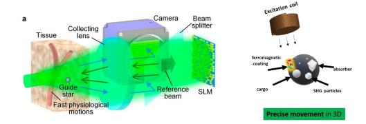
Left: DOPC setup with SHG Guide star inside tissue [1]. Right: Micro robot with SHG nanocrystal \_\_\_\_\_
