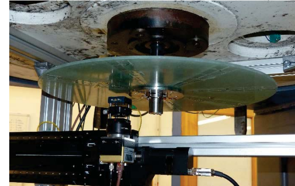
Optical sensor on FRP rotor inside test rig
