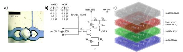
Figure: Chemofluidic circuit. A): Chemofluidic volume phase-transition transistor (CVPT), b): Circuit of the NAND or NOR gates based on a planar CVPTs, c): Microfluidic multi-layer concept for a multi-layer reactor chip.
