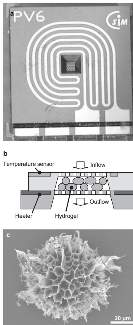
**Figure 1.** The chemostat design. a) The photograph of the chemostat shows the silicon-based upper plate, including the structure of the temperature sensor and the perforated membrane of the inflow. The dimension of the silicon chip is 5 mm  $\times$  5 mm. b) This schematic representation describes the internal structure of the chemostat. c) The microgel particles prepared by inverse-suspension polymerization are regular in shape and highly porous.
