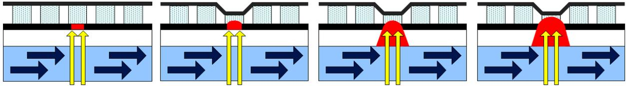
**Fig. 3. Functional principle of thermal control.** 1) start of heating, 2) actuation, 3) heat spreading, 4) steady state
