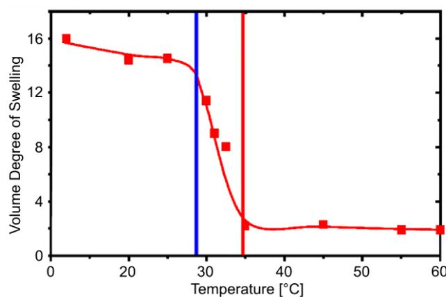
Fig. 2. Illustration of volume phase transition of the “smart hydrogel” PNIPAAm actuator.
