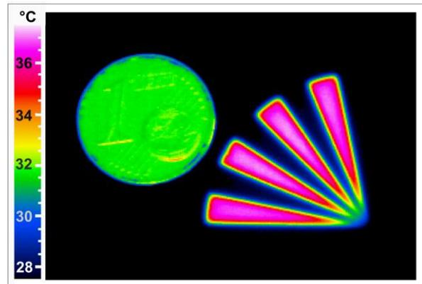
**Fig. 4. Response time of the thermal control unit and high resolution temperature image.**
