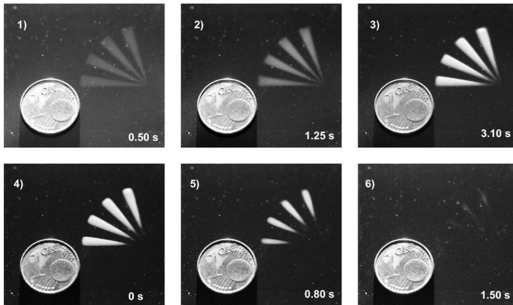
**Fig. 5. Generation of a monochrome image due to an applied temperature change.**
