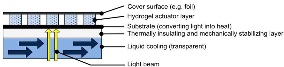
Fig. 1. Scheme of thermal control setup.
