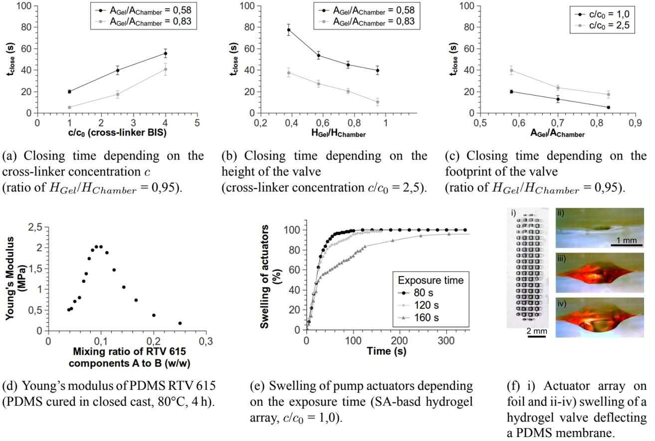
Fig. 2: Properties of the active elements used as closing valves and micropumps based on SA (exposure time for closing valves: 7 min).
