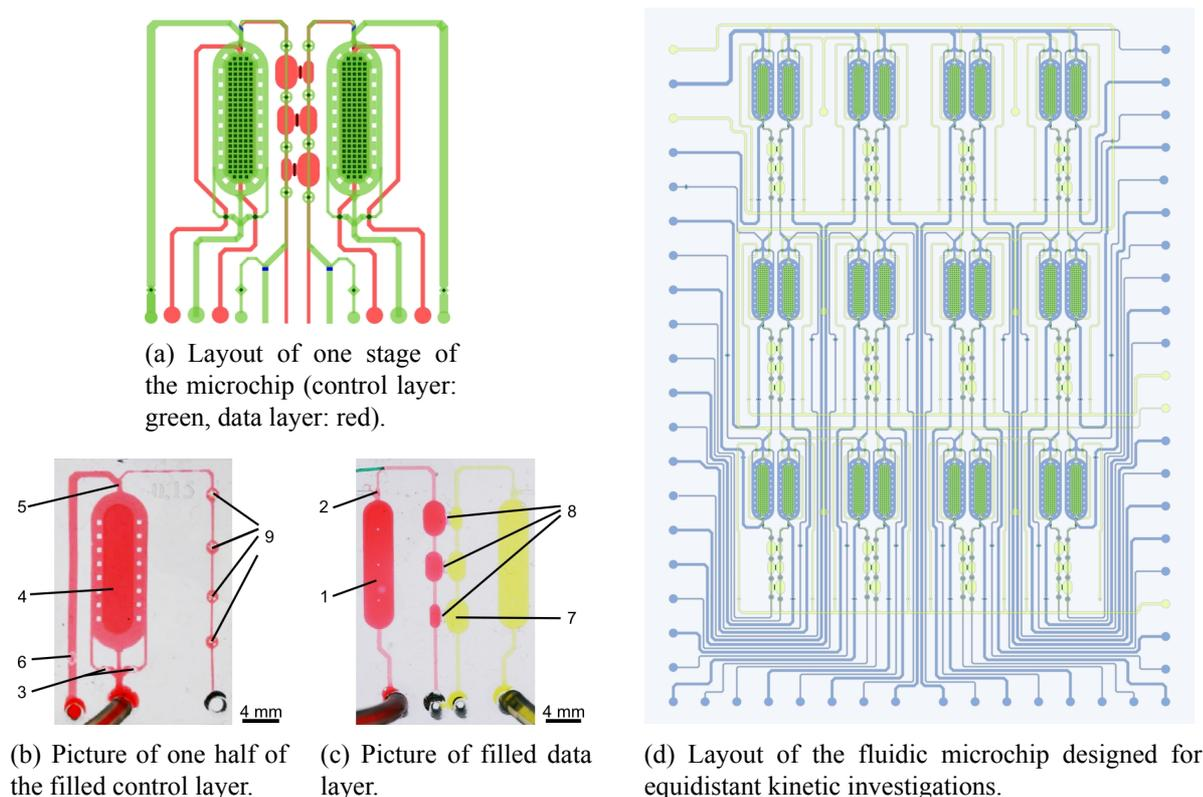
Fig. 3: Design of the microchip. For facility of inspection, in 3(b) and 3(d) control and data layer are shown separately.
