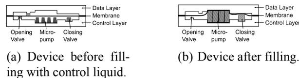
Fig. 1: Schematic cross section of the microchip.
