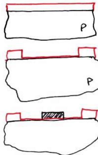
We start with the "field Oxidized" Wafer
