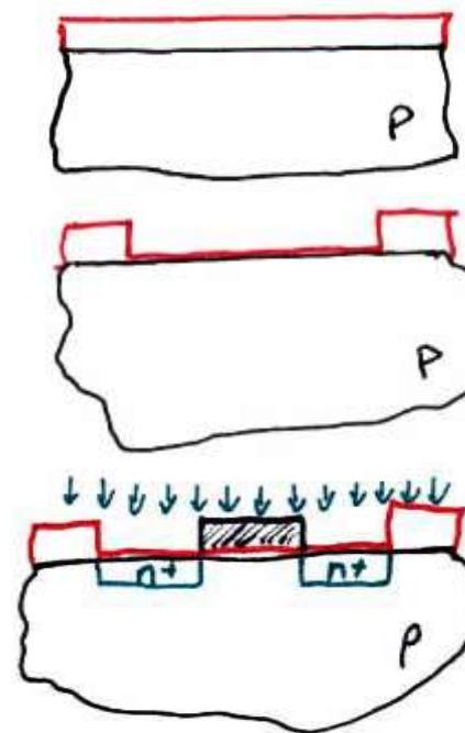
We start with the "field Oxidized" Wafer
