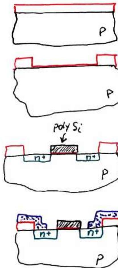
We start with the "field Oxidized" Wafer
