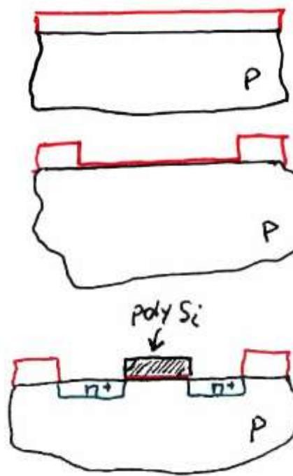
We start with the "field Oxidized" Wafer
