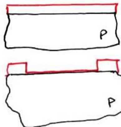
We start with the "field Oxidized" Wafer
