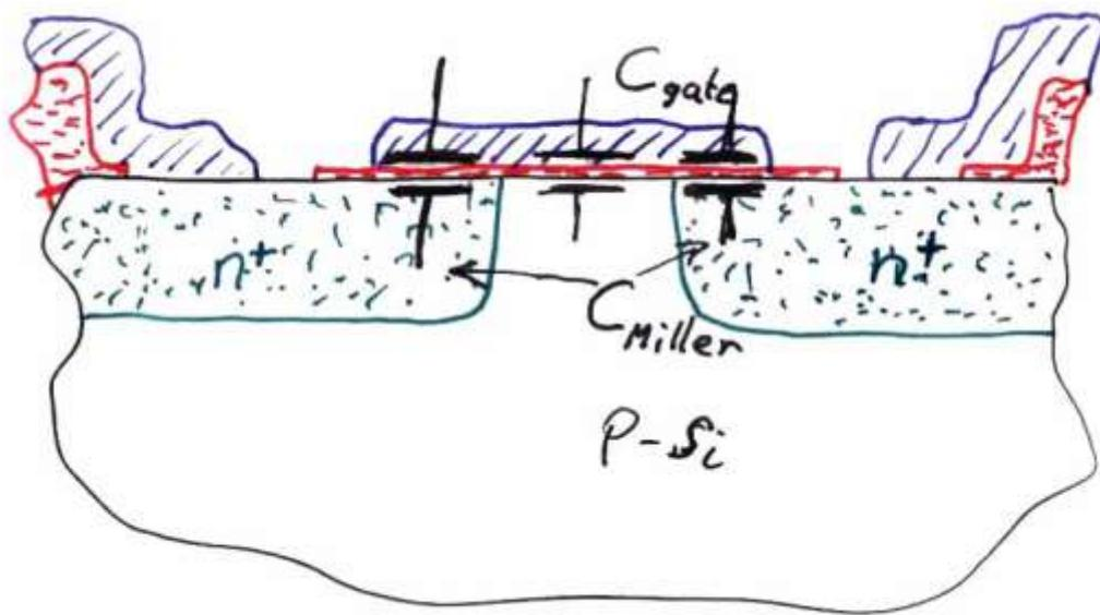
The Gate capacity determined by the charge to form the inversion channel
