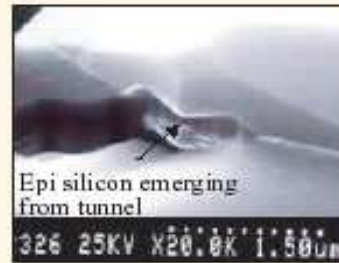
Grow selective epitaxial Si from one side of the tunnel
