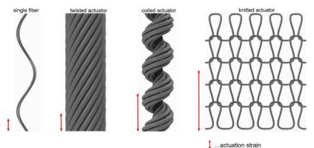
Schematic representation of potential textile structures to determine the relation between fiber- and textile structure and actuator performance, targeting an actuator performance enhancement for use in I-FRC.
