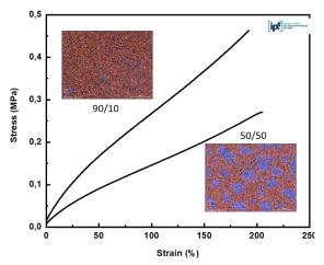
SEM-EDX images and stress-strain response of elastomers having liquid isoprene rubber (LIR-403 from Kuraray) and epoxy crosslinker (Polydis 3616 from Struktol) in 90/10 and 50/50 ratio
