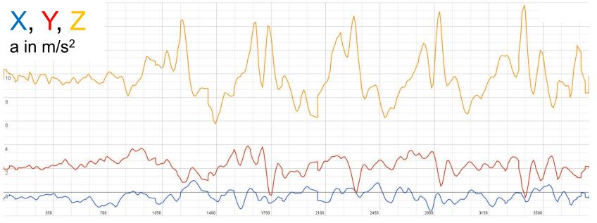
accelerometer data record of a walk
