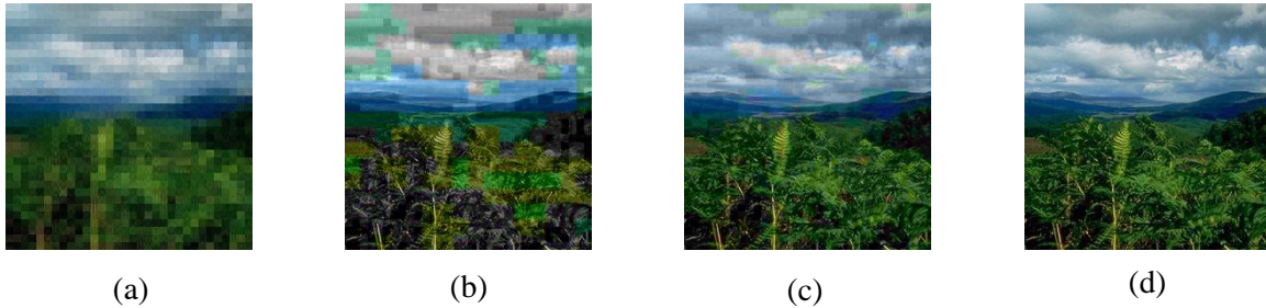
Figure 4.4 Results of using JPEG encoding after prediction. (a) The re-assembled image from coefficient differences that is sent to the JPEG encoder. (b-d) Decoded images for different quality levels (b) 1 (c) 15 (d) 100.
