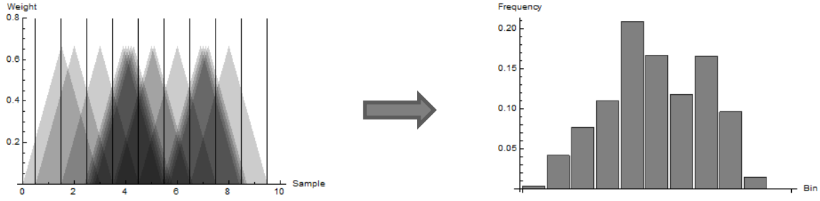
Figure 4.9 Adapted frequency calculation for entropy loss. Left: Sample distribution for triangle window; each peak represents a single sample's weight. Right: the resulting frequencies for each bin.
