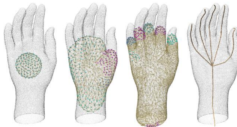
Figure 2: The deformable model with competing fronts. The fronts move in a coarse to fine manner, and may split to form sub-fronts, inducing the branching structure of our skeleton.
