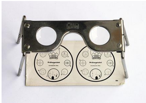
Pocket stereoscope with original test image. Used by military to examine stereoscopic pairs of aerial photographs.
