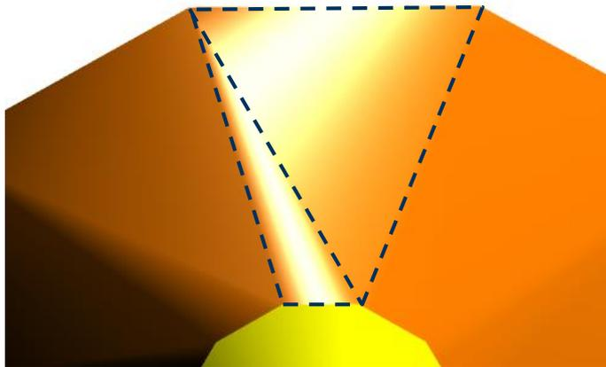
Illumination artefacts due to splitting of quad into badly shaped triangles
