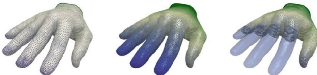
Fig. 2.9 Example of PL scalar field f defined on a PL 3-manifold \mathcal{M} . From left to right: restriction \hat{f} of f on the 0-simplices of \mathcal{M} , f (the color coding denotes the linear interpolation within each simplex), clipped view of f
