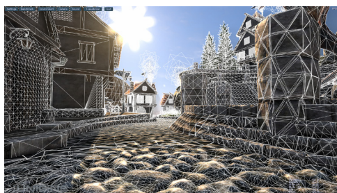
Figure 1: Tessellation of an object with different tessellation factors in relation to the cameradistance.
