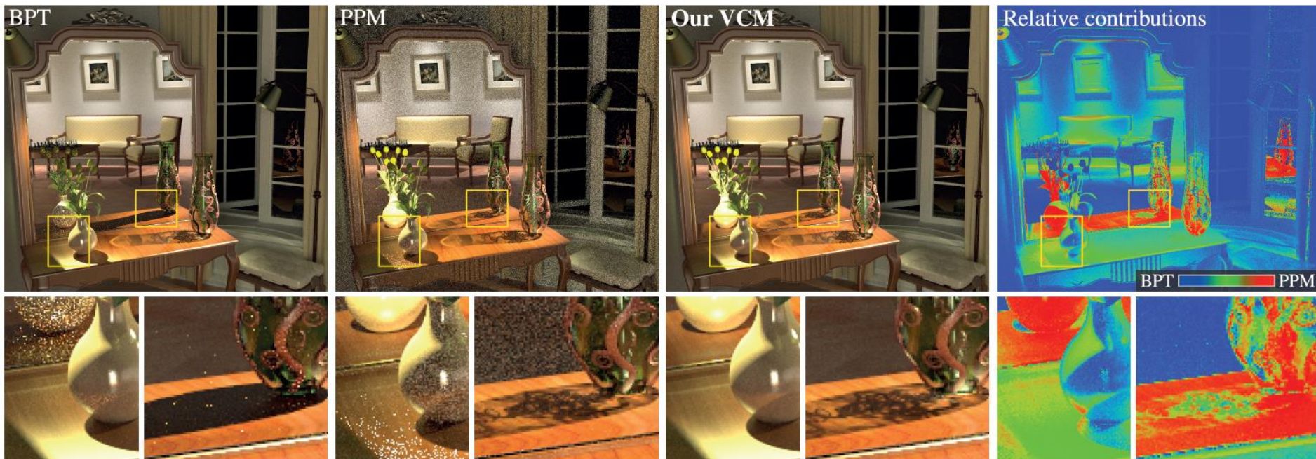
Figure 1: A comparison of our new progressive vertex connection and merging (VCM) algorithm against bidirectional path tracing (BPT) and stochastic progressive photon mapping (PPM) after 30 minutes of rendering. BPT fails to reproduce the reflected caustics produced by the vase, while PPM has difficulties in handling the illumination coming from the room seen in the mirror. Our new VCM algorithm automatically computes a good mixture of sampling techniques from BPT and PPM to robustly capture the entire illumination in the scene. The rightmost column shows the relative contributions of the BPT and PPM techniques to the VCM image in false color.
