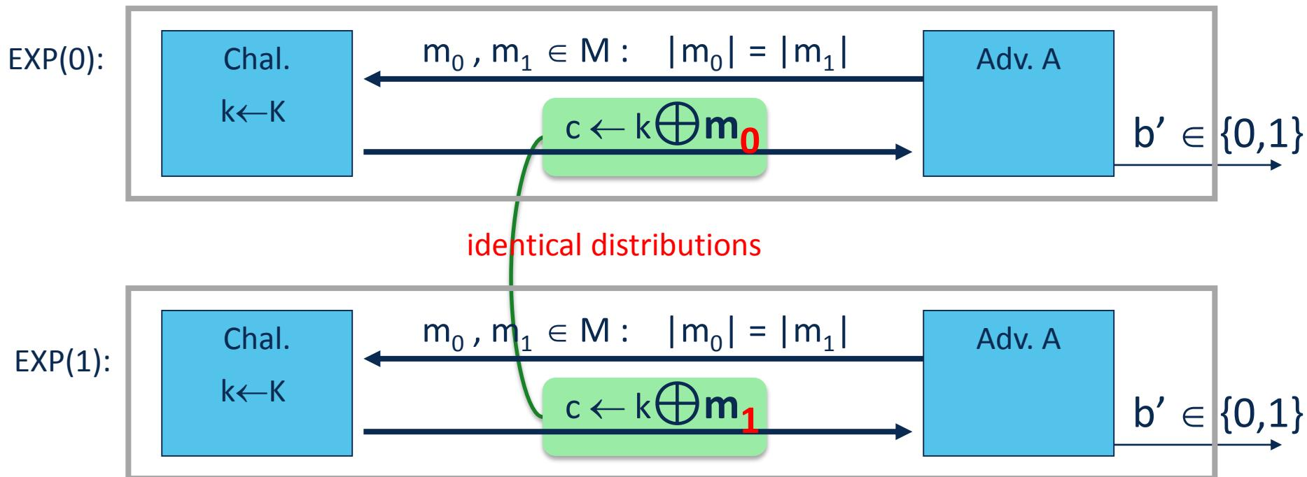
For all A:  $\text{Adv}_{\text{SS}}[\text{A}, \text{OTP}] = \left| \Pr[\text{A}(k \oplus m_0) = 1] - \Pr[\text{A}(k \oplus m_1) = 1] \right|$
