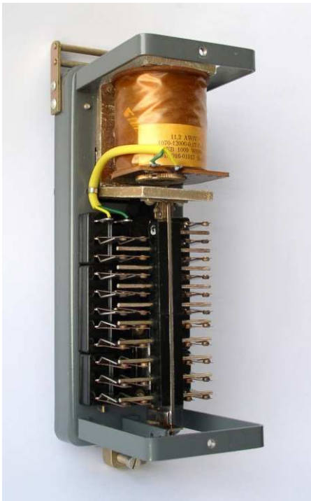
Normalrelais, Bauform II (WSSB) [2]
