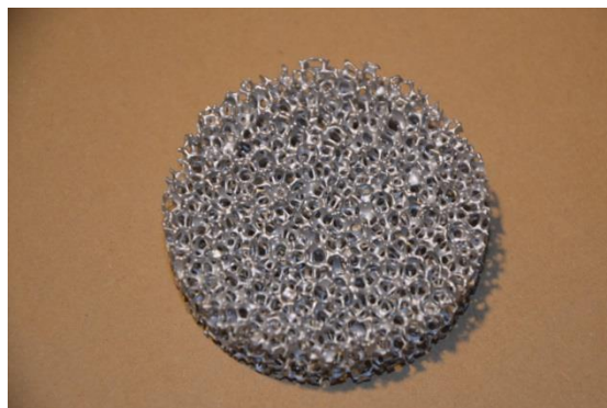
Figure 1 Metal Foam (10 ppi, stainless steel, Fraunhofer IFAM)
