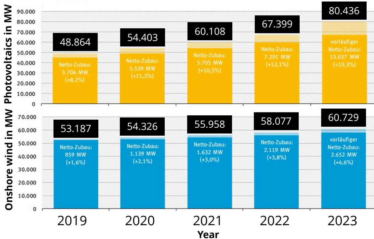
Development of the installed power of PV and onshore wind in Germany [1]
