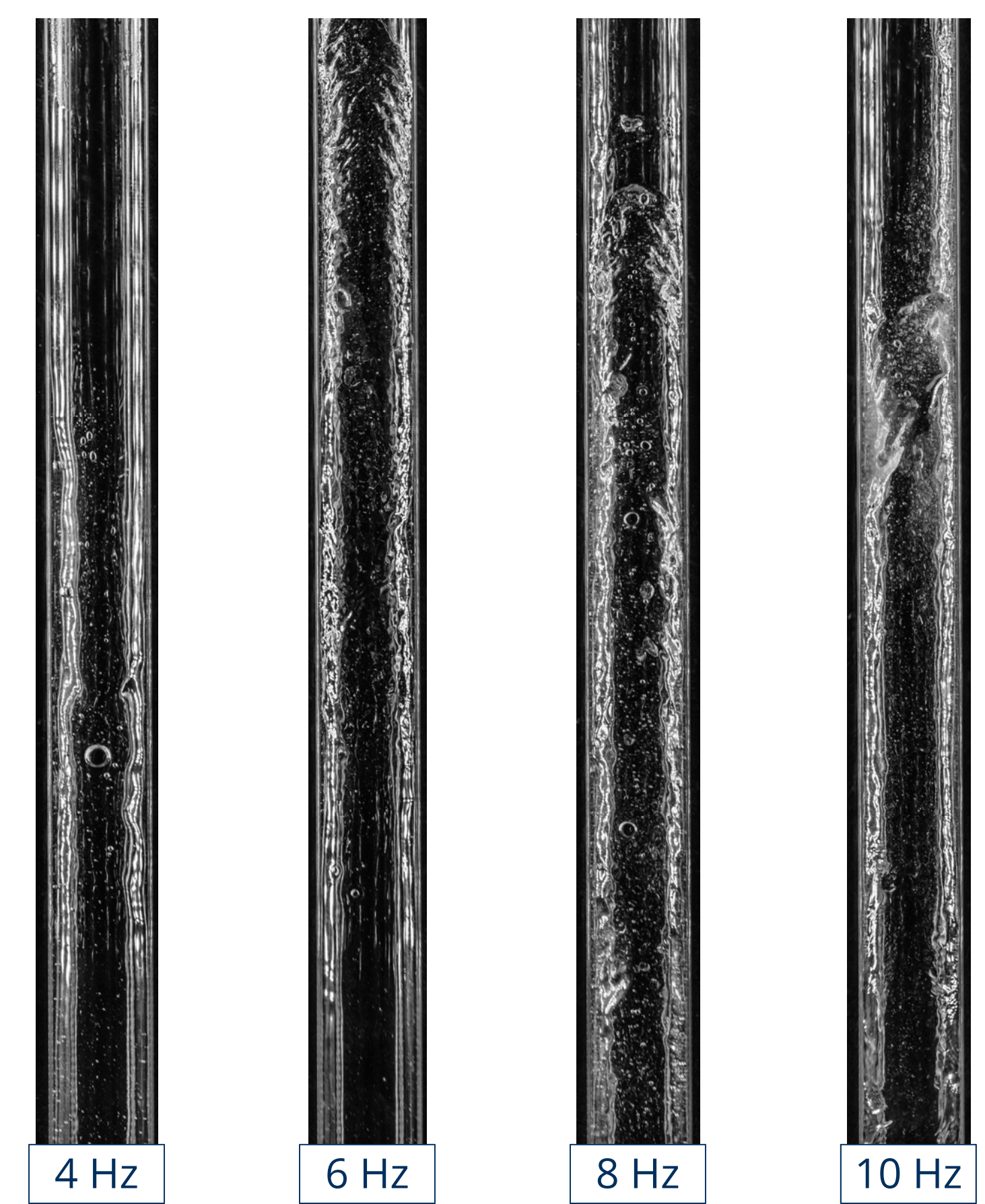
Fig. 3: Different flow characteristics inside the reciprocating glass pipe for different oscillation frequencies
