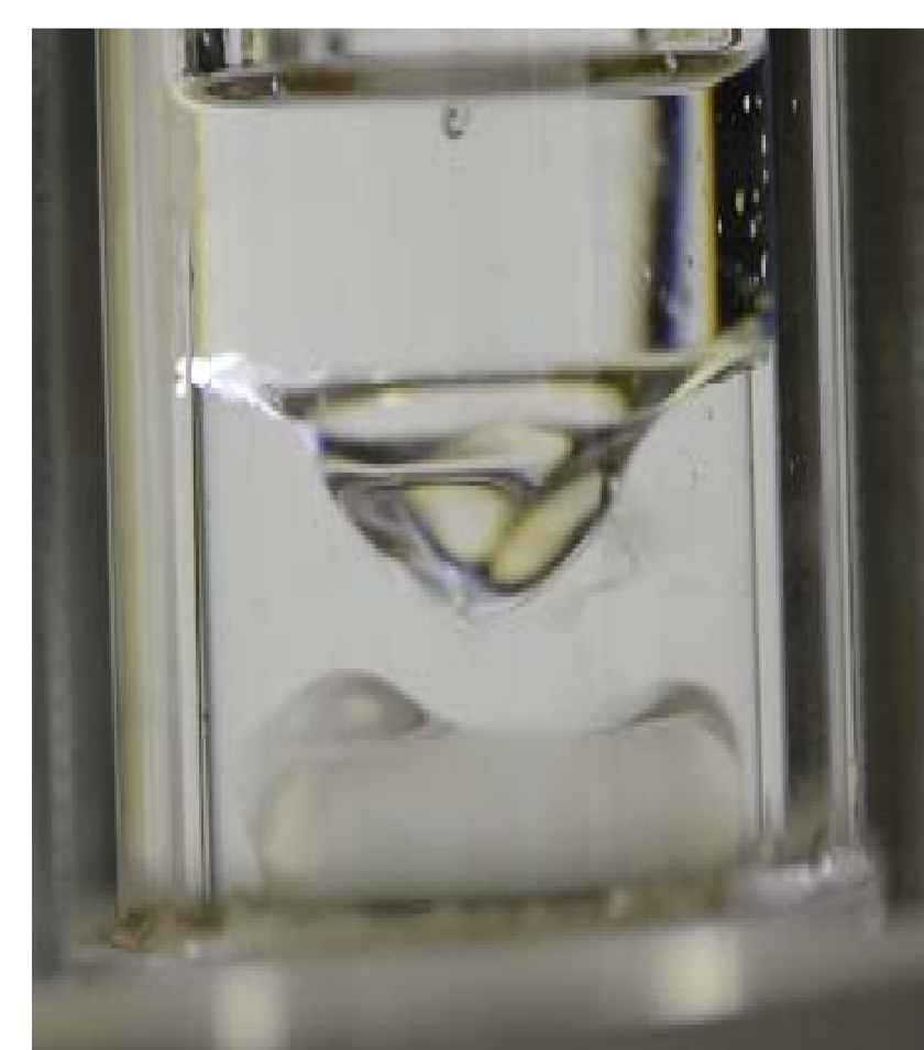
Fig. 3: left: Incremental appearance of a miscibility gap of R744 and a POE, right: Miscibility gap of ammonia and a mineral oil
