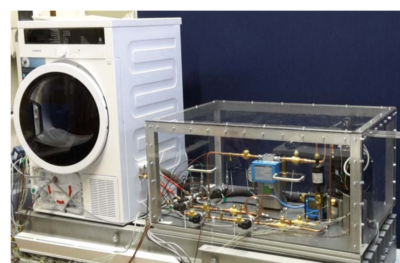
Fig. 4: Heat Pump Tumble Dryer Test Rig
