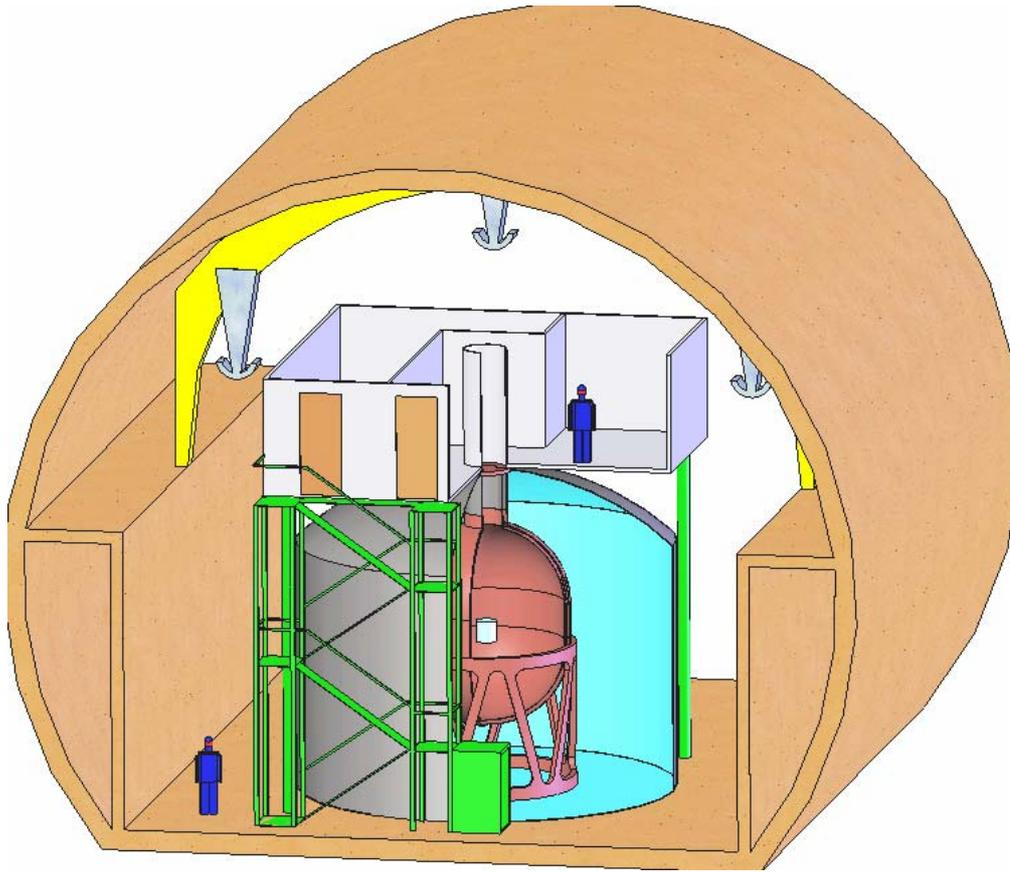
**FIGURE 2.** Artist's view of the GERDA set-up in the Gran Sasso underground laboratories (LNGS) in Assergi, Italy. The 70 m<sup>3</sup> cryostat with the diode arrays suspended in its center is placed inside a water tank. On top of the cryostat are mounted the lock and cleanrooms..
