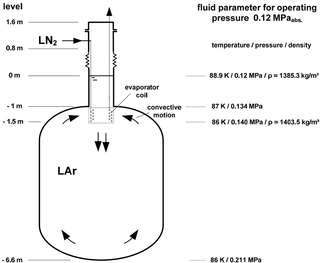
**FIGURE 4.** Pressure and temperature levels inside the 70 m<sup>3</sup> LAr cryostat due to active cooling and hydrostatic pressure, with convective flow in the main volume.
