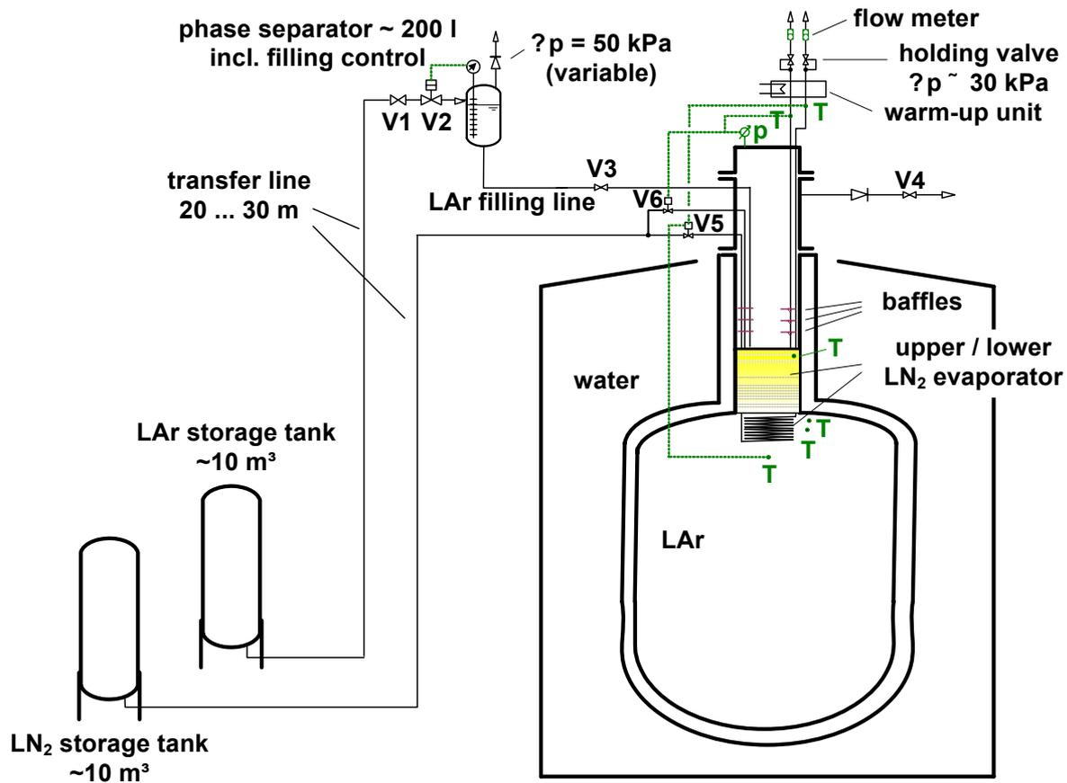
**FIGURE 3.** Simplified flow scheme of the cryogenic supply of the GERDA cryostat. T and p denote locations for temperature and pressure sensors, respectively. Control loops are indicated by dashed lines.
