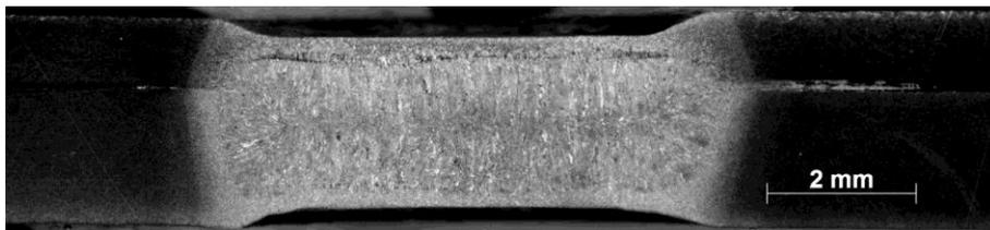
Abbildung 111: Querschliff der Schweißprobe 7M\_I12,0kA\_P0001,  $I_w = 12,0$  kA,  $F_e = 3,0$  kN,  $t_w = 200$  ms
