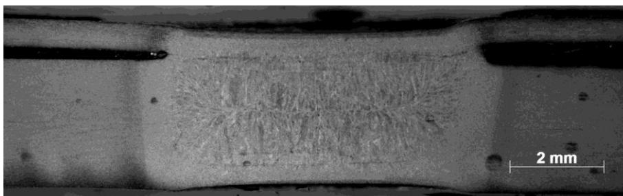
Abbildung 46: Querschliff der Schweißprobe 1RSW\_I8,0kA\_P0004,  $I_w = 8,0$  kA,  $F_e = 2,0$  kN,  $t_w = 600$  ms
