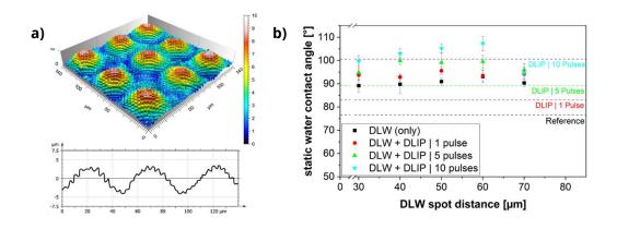
(a) Confocal images and extracted profiles of a hierarchical structured PET film consisting of a DLW structure with diameter 50  $\mu$ m at a height of 8  $\mu$ m combined with a 3.1  $\mu$ m periodic DLIP structure with a height of 1.8  $\mu$ m. (b) Results of static water contact angle measurements as a function of DLW structure spacing for different texture combinations compared to the unstructured reference surface (black)
