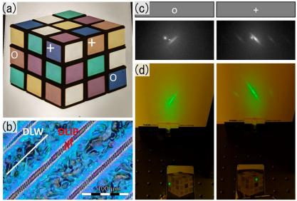
Photograph of colorized motive with hidden security features (a); optical microscopy image of the DLW-treated lines and DLIP-structure orientation (b); monitoring system images taken from a field with DLIP-structures "+" and from a featureless field with the same color "O" (c). Photographs of diffraction patterns projected on a screen from the corresponding fields labeled as "O" (left) and "+" (right) and upon being illuminated with a laser pointer (d).
