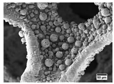
SEM image of structured open cell metal foam, spatial period 5.8  $\mu m$ , line-like patterning.
