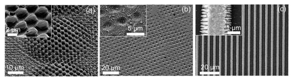
SEM images of patterned (a) PET with pillar-like array, (b) sodalime glass with hole-like texture and (c) ITO film with line-like grooves.
