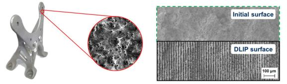
Example of additive manufactured 3D component and exemplary SEM images of the surface topography before and after direct laser interference patterning.
