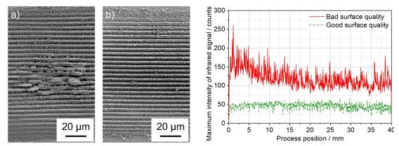
SEM images of structured stainless steel samples in a bad (a) and good surface condition (b) and corresponding maximum intensity of the infrared signal captured by the infrared camera as function of the process position during the laser treatment representing the different surface conditions.
