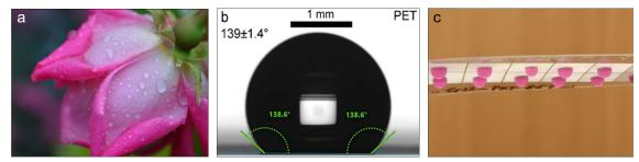
Fig. 1(a) Optical image of water droplets on rose petals. (b) WCA on the patterned PET surface. (c) Photographs of water droplets (dyed by 0.1% KMnO4 solution) on PET film with a tilting angle of 180°.
