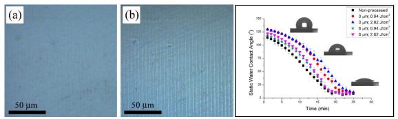
Bright field (a) and phase contrast (b) images of DLIP structured PHEMA, and time-dependent static water contact angle measurements performed during the absorption of the water droplet by the polymer samples
