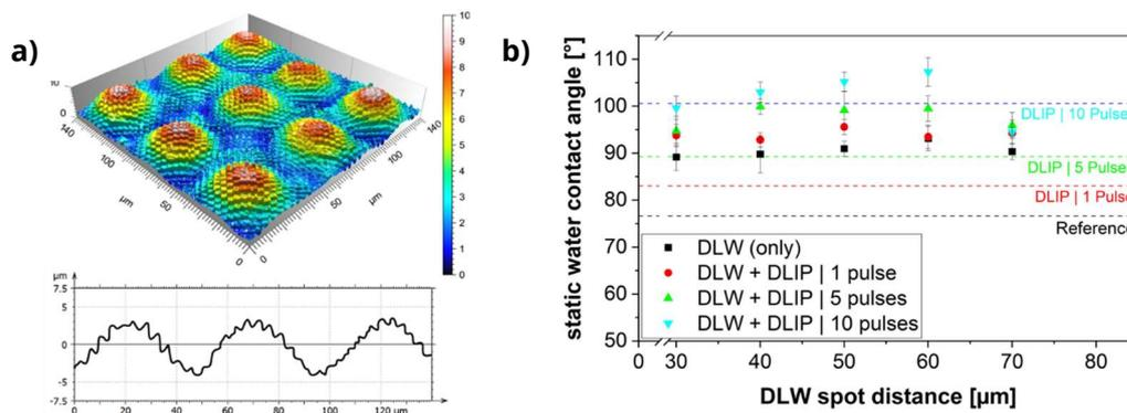
(a) Confocal images and extracted profiles of a hierarchical structured PET film consisting of a DLW structure with diameter 50  $\mu\text{m}$  at a height of 8  $\mu\text{m}$  combined with a 3.1  $\mu\text{m}$  periodic DLIP structure with a height of 1.8  $\mu\text{m}$ . (b) Results of static water contact angle measurements as a function of DLW structure spacing for different texture combinations compared to the unstructured reference surface (black)
