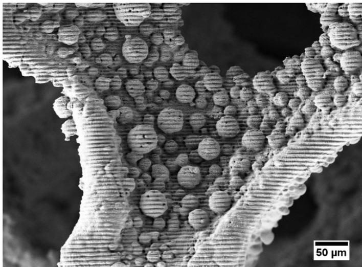
SEM image of structured open cell metal foam, spatial period 5.8 $\mu\text{m}$ , line-like patterning.
