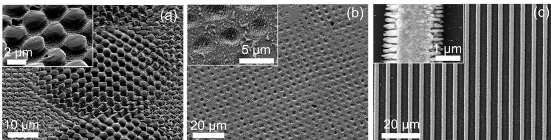
SEM images of patterned (a) PET with pillar-like array, (b) sodalime glass with hole-like texture and (c) ITO film with line-like grooves.
