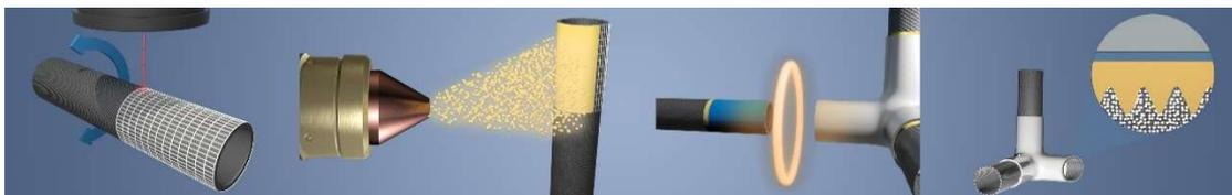
Schematic process chain (f.l.t.r.): Laser pre-treatment, thermal spray coating, soldering and a materially bonded multi-material joint © Fraunhofer IWS
