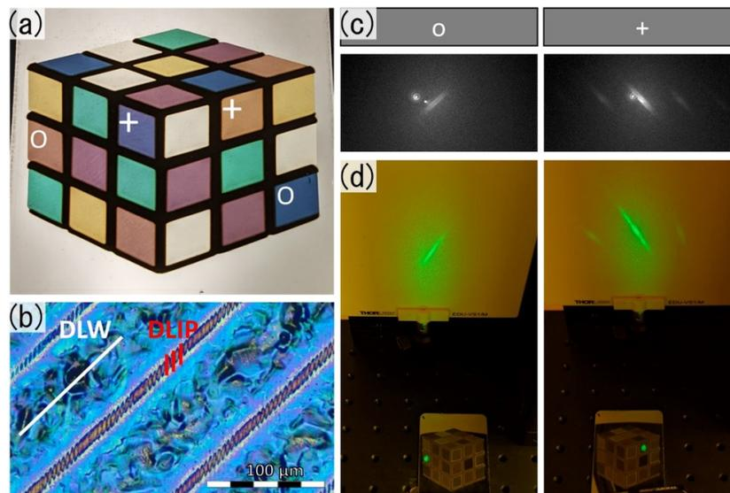
Photograph of colored motive with hidden security features (a); optical microscopy image of the DLW-treated lines and DLIP-structure orientation (b); monitoring system images taken from a field with DLIP-structures “+” and from a featureless field with the same color “O” (c). Photographs of diffraction patterns projected on a screen from the corresponding fields labeled as “O” (left) and “+” (right) and upon being illuminated with a laser pointer (d).
