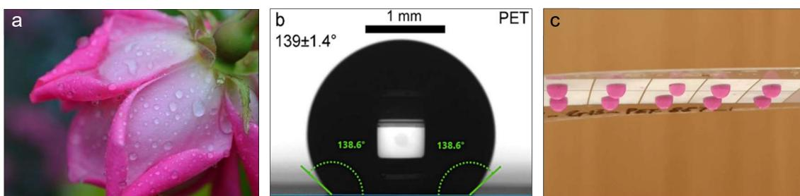
Fig. 1(a) Optical image of water droplets on rose petals. (b) WCA on the patterned PET surface. (c) Photographs of water droplets (dyed by 0.1%  $\text{KMnO}_4$  solution) on PET film with a tilting angle of  $180^\circ$ .
