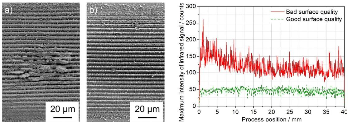
SEM images of structured stainless steel samples in a bad (a) and good surface condition (b) and corresponding maximum intensity of the infrared signal captured by the infrared camera as function of the process position during the laser treatment representing the different surface conditions.
