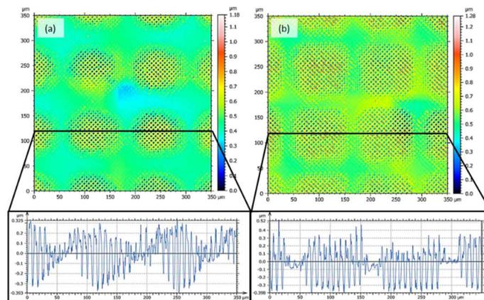
Confocal microscope images of surface topographies produced on stainless steel and corresponding surface profiles using the (a) Gaussian and (b) top-hat beam profiles. Only one laser pulse was used for each spot. The laser fluence was  $2.97\text{ J/cm}^2$  and the hatch distance was  $130\mu\text{m}$ .
