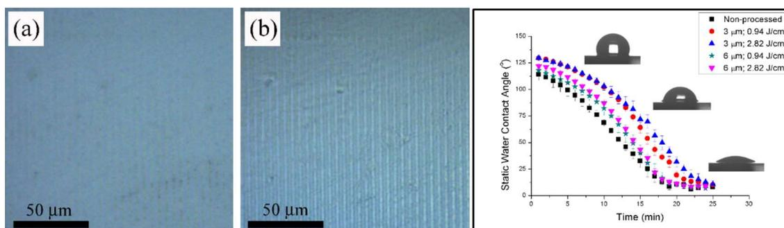
Bright field (a) and phase contrast (b) images of DLIP structured PHEMA, and time-dependent static water contact angle measurements performed during the absorption of the water droplet by the polymer samples
