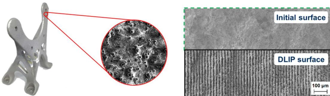
Example of additive manufactured 3D component and exemplary SEM images of the surface topography before and after direct laser interference patterning.
