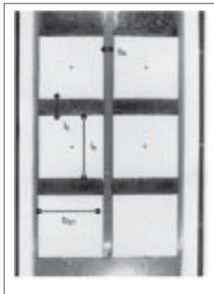
»6 Block setting in the water channel [2]
