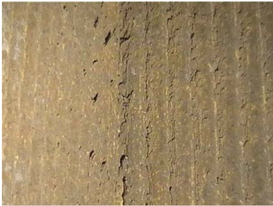
a) membrane wall without lining, with deposits
