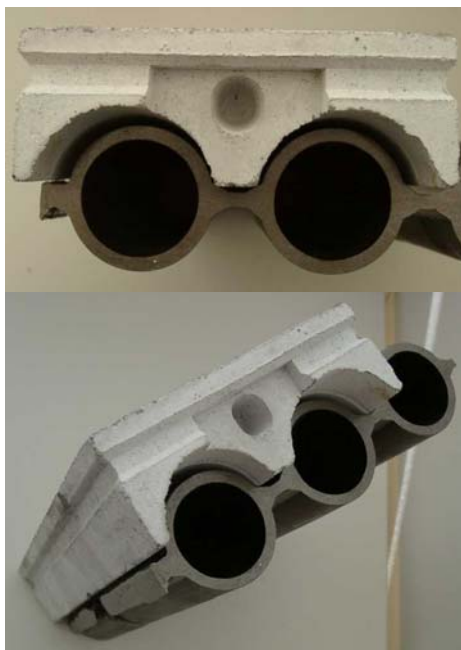
Fig. 2. Real system, Jusys4-tile with part of membrane wall.
