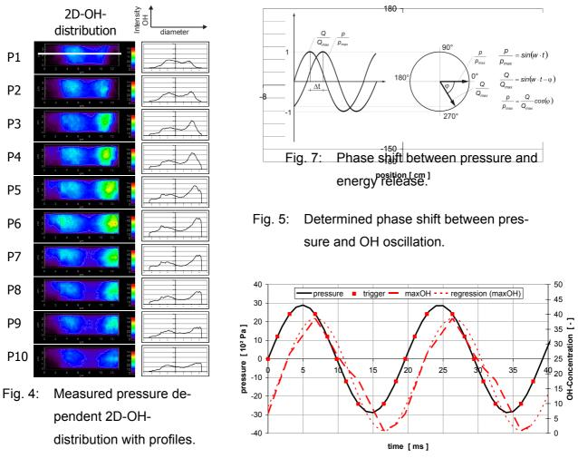
Fig. 6: Phase shift between pressure oscillation and maximal OH-concentration.
