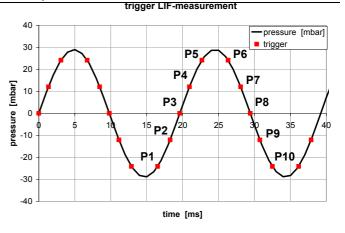
Fig. 2: Schematic illustration of pressure measurement points for LIF measurement.
