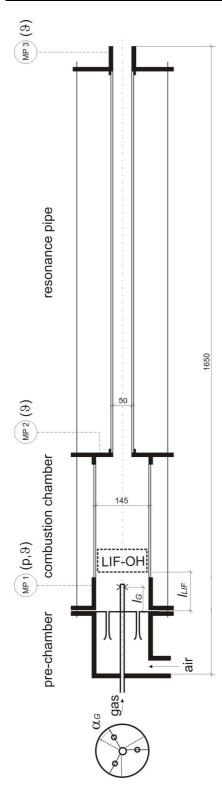
Fig. 1: Schematic diagram of the model of the Pul-sations-reactor.
