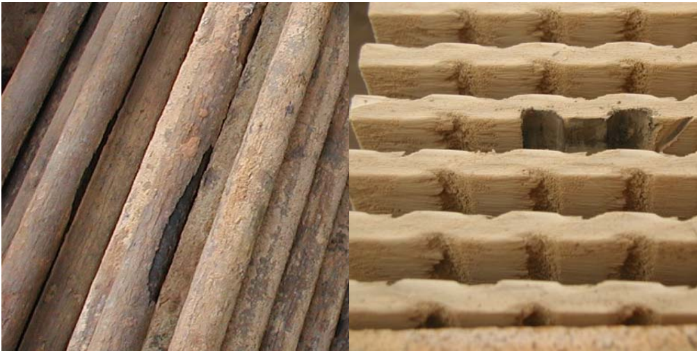
Figure 4: Tube bundle heat exchanger and heat exchanger from ceramics after a short operation time
